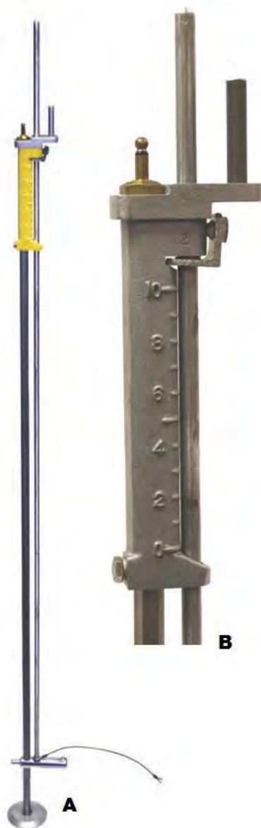
Fig. 2. A. The complete assembled wading rod. B. The Vernier scale.
